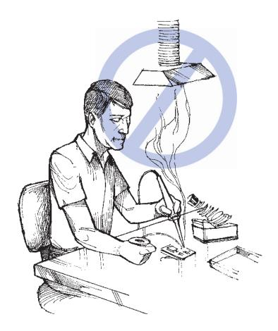
This is the wrong position for an exhaust hood. Ventilation must not draw lead fume or dust past the worker's breathing area.
