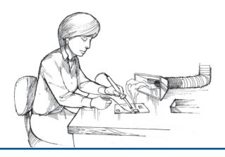
Ventilation should draw lead fume or dust away from the work and the worker.
