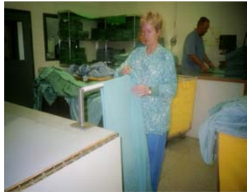
Figure 4. After changes, a "gurney guy" clamps to the table to eliminate holding.
