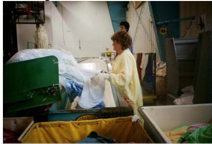
Figure 2. “Dumper” shows an extended conveyor with higher sides and plastic bags that reduce awkward dumping postures.
