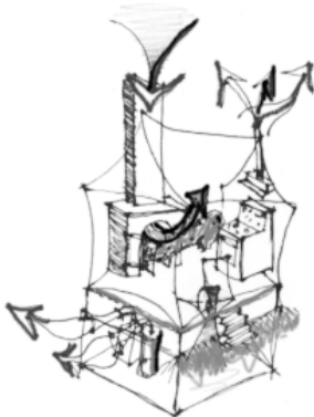
Figure 14: Negative pressure within a home.
