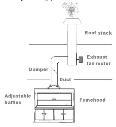
The speed of the air moving through the hood opening is known as face velocity. This laboratory worker guide is intended to help identify fume hood types and outline exposure control practices in relation to the fume hood.
