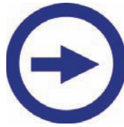
FIGURE 2-42 STANDARD SYMBOL DESIGNATING FORCED TO BREAK CONTACT DEVICES
