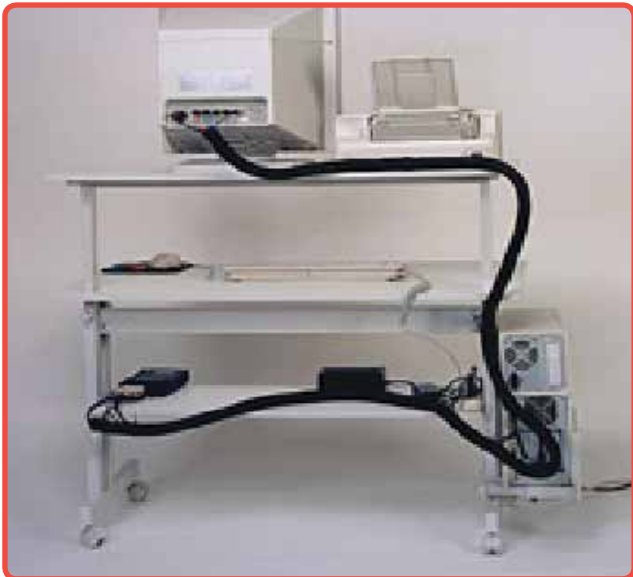
Figure 9.9. Plastic outer sleeve that covers the loose cords (i.e., cord organizer)
