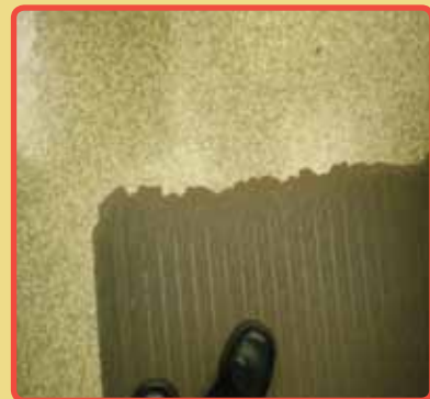
Figure 10.2. Frayed, worn edges on a comfort mat
