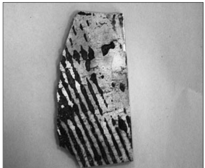
Vinyl asbestos flooring
